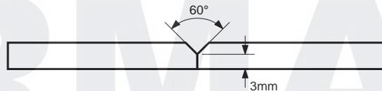
(EN) Preparation of the edges for butt weld joints to be welded with weld material.
